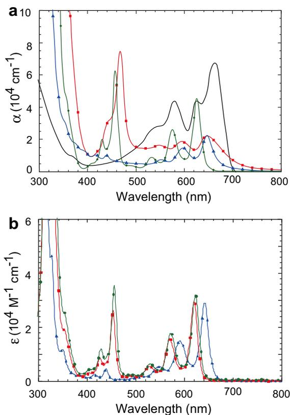
**Fig. 2.** (a) Thin-film extinction spectra of the pentacene derivatives TIPS (green, circles), TP-5 (red, squares), and EtTP-5 (blue, triangles). The extinction spectra of pentacene is shown for comparison (black line). (b) Solution extinction spectra of TIPS (green, circles), TP-5 (red, squares), and EtTP-5 (blue, triangles). (For interpretation of the references to colour in this figure legend, the reader is referred to the web version of this article.)
