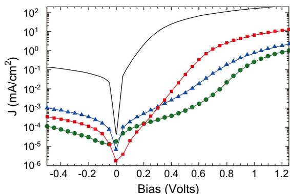
**Fig. 3.** Dark current density–voltage characteristics for the pentacene/ $C_{60}$  (black line) and derivative/ $C_{60}$  photovoltaic cells [TIPS (green, circles), TP-5 (red, squares), and EtTP-5 (blue, triangles)]. (For interpretation of the references to colour in this figure legend, the reader is referred to the web version of this article.)
