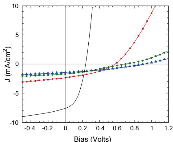
**Fig. 4.** Illuminated  $J$ - $V$  characteristics (AM1.5,  $100 \text{ mW}/\text{cm}^2$ ) for the pentacene/ $C_{60}$  (black line) and derivative/ $C_{60}$  photovoltaic cells [TIPS (green, circles), TP-5 (red, squares), and EtTP-5 (blue, triangles)]. (For interpretation of the references to colour in this figure legend, the reader is referred to the web version of this article.)
