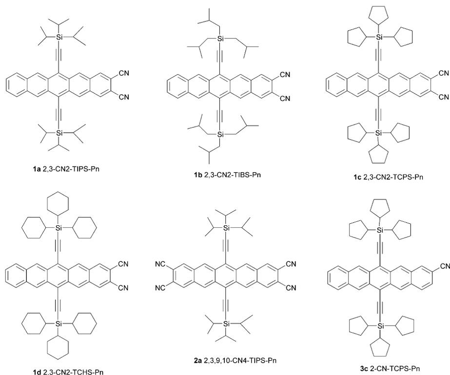
**Fig. 2** Molecular structures of the cyanopentacenes.
