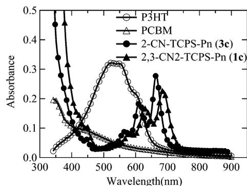
**Fig. 8** UV-Vis absorption spectra comparison between P3HT, PCBM, and the best performing cyanopentacene derivatives.
